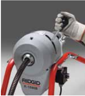
Engage clutch, cable spins
