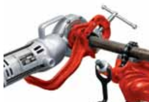
Threading using a pipe wrench as a support arm
