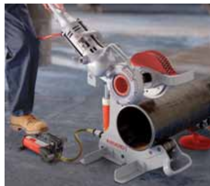
Model 258 Pipe Cutter with No. 700 Power Drive in use for cutting
